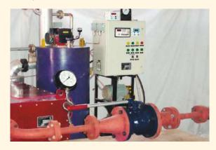
Microfinish research and development facilities include high temperature test loop to 480 °C (896 °F) at 15 bar pressure
